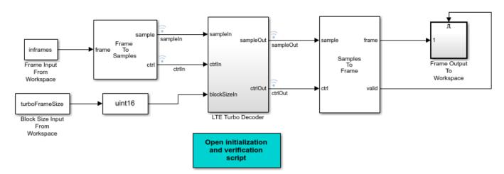
The **LTE Turbo Decoder** subsystem consists of the LTE Turbo Decoder block. This block is set to run for a frame size of 6144 systematic bits and 6 iterations of decoding.
