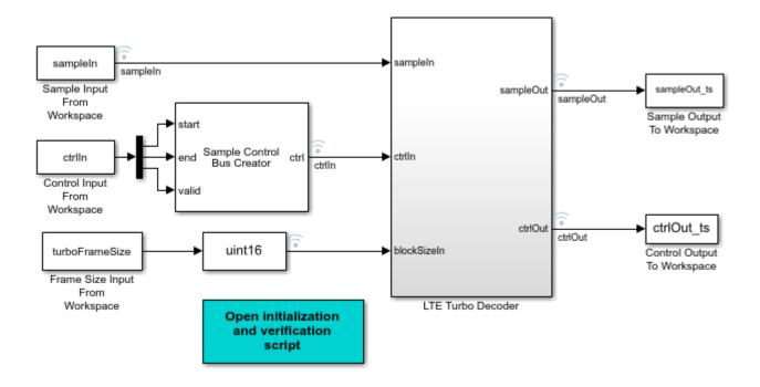
The **LTE Turbo Decoder** subsystem consists of the LTE Turbo Decoder block. This block is set to run 6 iterations of decoding.
